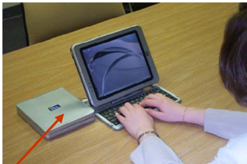
10.5 V, 50 WH Battery utilizing 250 WH/kg prototype cells, discreet electronic components & machined plastics!
